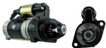
ARRANQUE MINXIAN QDJ1409E-P 12v. Z11 3.8kw PALA MICHIGAN
