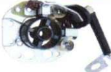
Porta Carbon Tipo COMSTAR 233004485R RENAULT DUSTER KWID SANDERO
